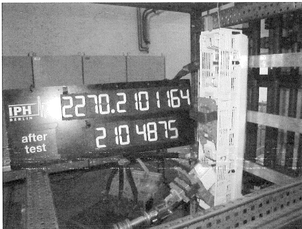
Photo 5: Test object L3 after conditional short-circuit current test
